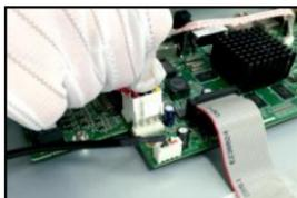
Figure 2-3 Connect Power Cable
